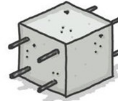
Reinforced Concrete** 635 kgCO 2 e/m 3
