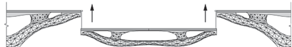
Step 4: Center part is lifted up and connected to both sides.
