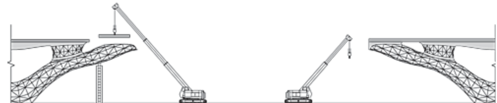
Step 2: Arch-Tube and Sandwich Roof Plate
