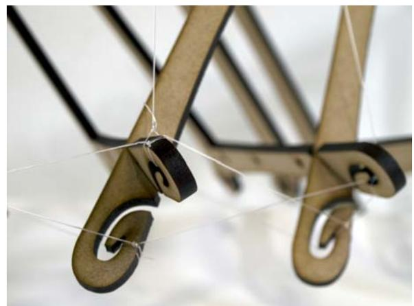
Figure 15. Tensegrity footbridge study – 1:20 scale model
