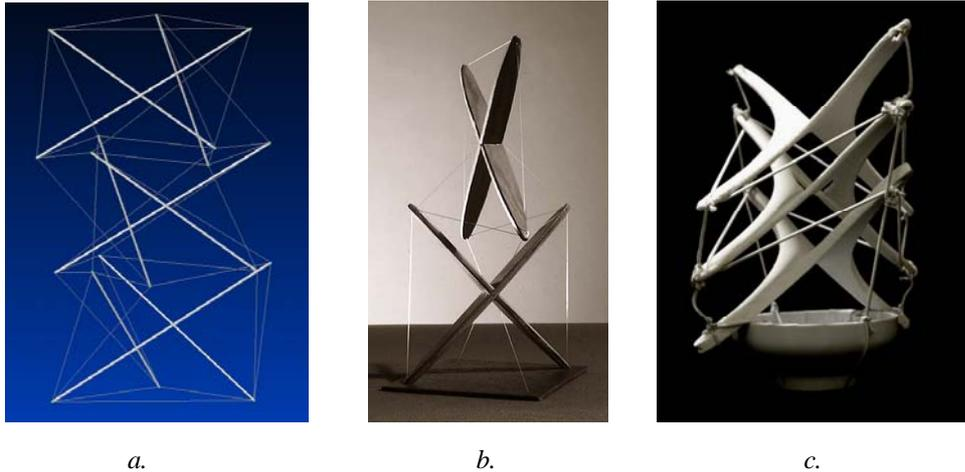
Figure 1. 1D bar, 2D X-shape and 3D tetrahedral tensegrity 'masts'
