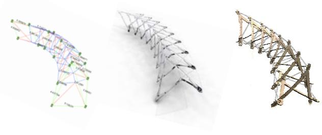
Figure 14. Comparison of computational, digital and physical models
