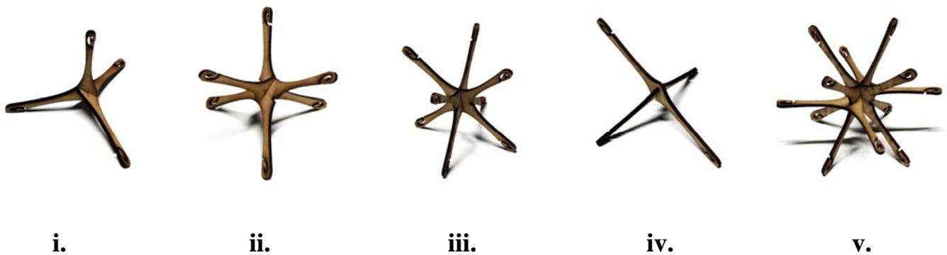
Figure 3. 3D components assembled using 2D laser cut pieces
