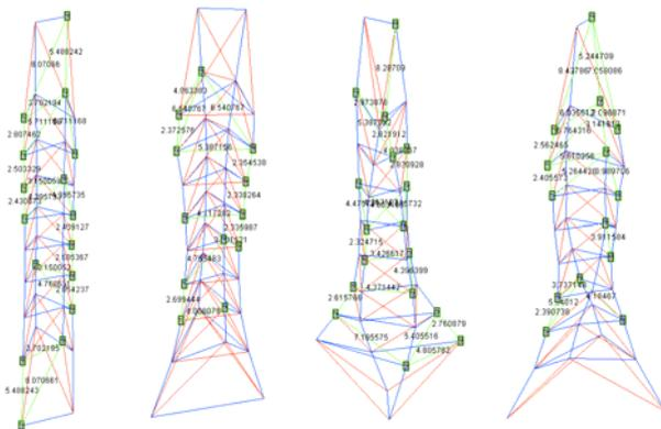
Figure 19. Computational form finding to explore alternate high-rise form
