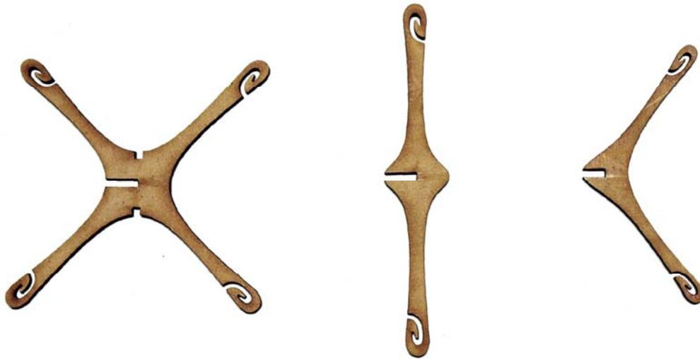
Figure 2. Laser cut parts for 3D components based on stable polyhedra: X-piece, Linear bar, and tetrahedral angle
