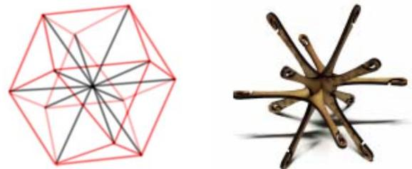
Figure 5. Cuboctahedron module and component
