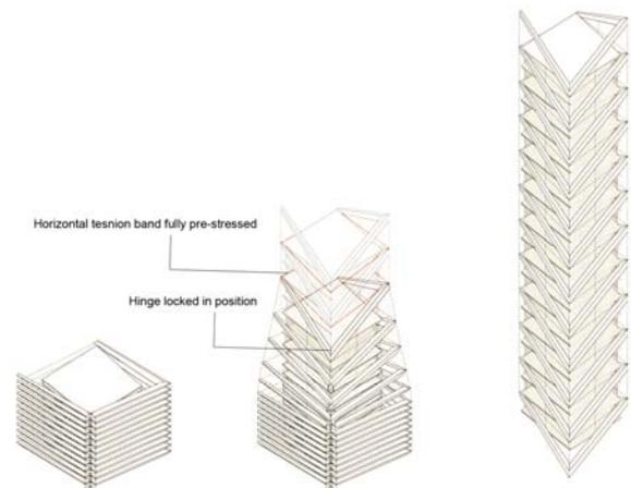
Figure 18. High rise deployment diagram
