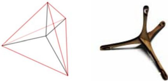
Figure 4. Tetrahedron module and component
