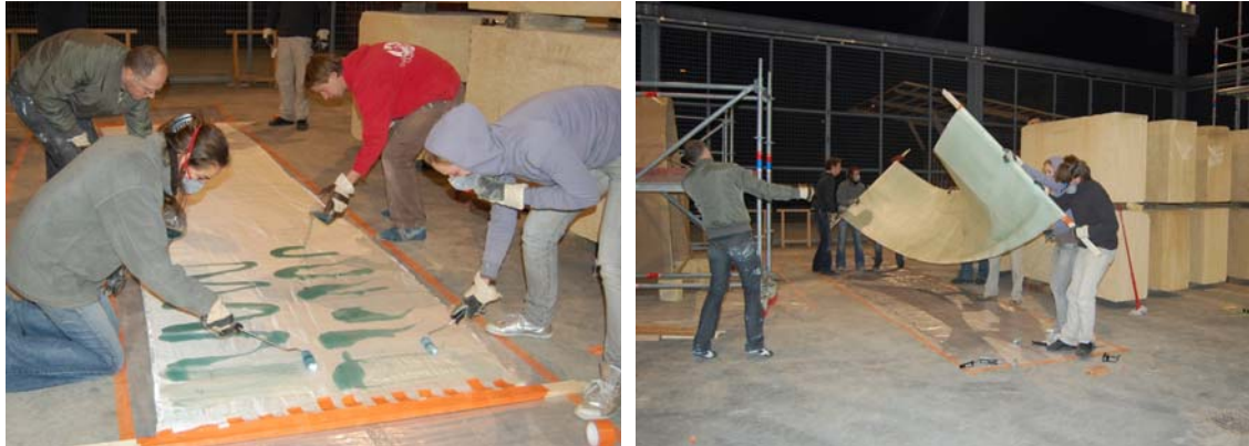
Fig.10 – Application of the resin on the weave
