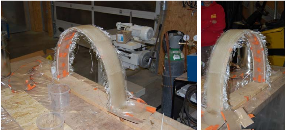
Fig.9 – Small scale models of the composite sandwich material
